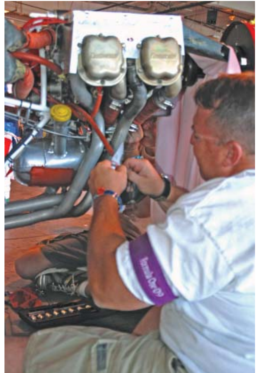
Greg repairs the #3 spark plug wire. The heat from the exhaust melted the top of the plug, but did no other damage to the engine.
