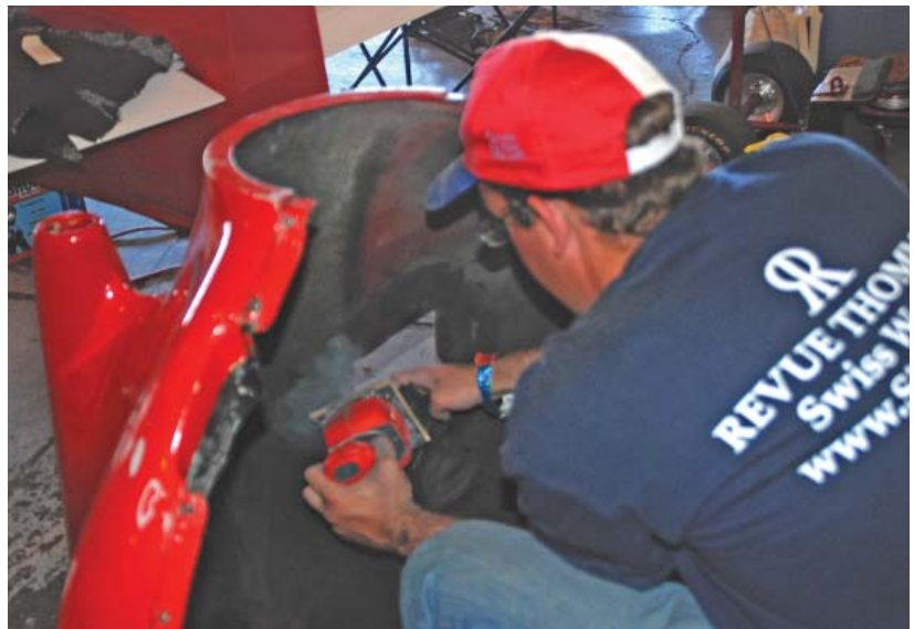
Steve Samuelian, from Smokey Young's crew, lays carbon fiber on the inside of the damaged cowling.
