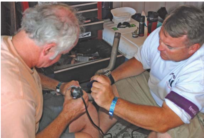
Greg holds while Gene uses a Dremel tool to smooth out the inside of the repaired pipe.
